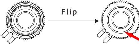
Rotating gobo 1 Gobo fixing seat
